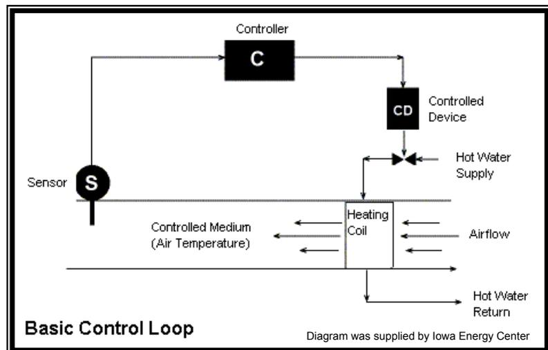
A control loop is the interaction between the sensors, the controller and the controlled devices. An example of a HVAC control loop would be indoor air temperature regulation. The sensor measures the indoor air
